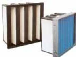
are available with a colorimetric efficiency from 50% to 98%, that is, from EU6/F6 a EU9/F9 according to Eurovent. The filters can be accessed for maintenance through a door with handle and hinges that normally allows removal upstream in the air flow.
